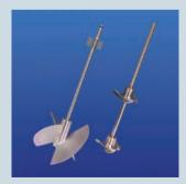
Optional impellers: Pitched blade impeller (left) for high aeration and low shear in insect and other cell cultures; marine blade impeller (right) for the growth of insect cells and other cultures
