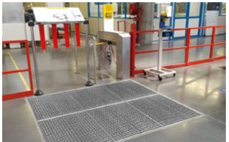
Cleaning of soles and rollers by ProfilGate® st55 go in front of the ESD-area
